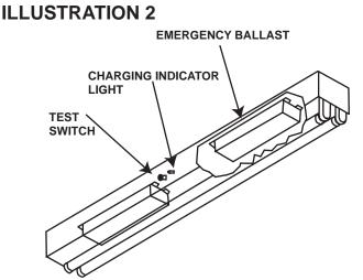
3. Install the test switch through the ballast channel cover of a troffer or through the side of a strip fix- ture. Drill a 1/2" hole and install the switch as shown. (See illustrations 1,2,& 3). Wire the test switch so that it removes AC power from both the emergency ballast and the AC ballast at the same time. (See illustration 5).
