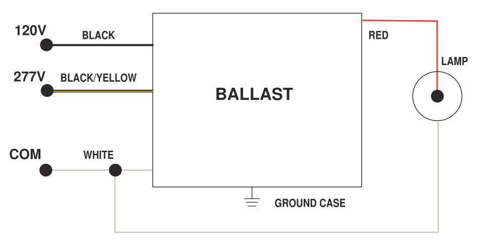
MINIMUM STARTING TEMPERATURE -20°F OR -30° C MAXIMUM BALLAST TO LAMP DISTANCE: 10 FEET INSULATE UNUSED INPUT LEAD FOR 300 VOLTS INSULATE LAMP LEAD CRIMP FOR 1000 VOLTS INSTALL IN ACCORDANCE WITH NATIONAL ELECTRICAL CODE
