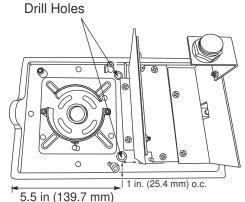
The backplate has a cast-in drill and knock-out template to match any standard recessed junction box
