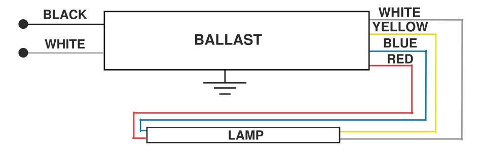
CAUTION: HIGH VOLTAGE: GROUND BALLAST CASE TO AVOID POSSIBLE SHOCK HAZARD. MOUNT LAMPS WITHIN 1/2 IN. OF GROUNDED METAL REFLECTOR.
