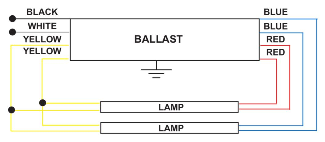
CAUTION: HIGH VOLTAGE: GROUND BALLAST CASE TO AVOID POSSIBLE SHOCK HAZARD. MOUNT LAMPS WITHIN 1/2 IN. OF GROUNDED METAL REFLECTOR.
