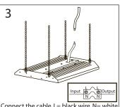
Connect the cable, L= black wire, N= white wire, G= green wire. Please keep the circuit open during the process.
