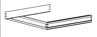
4.Choose the opening part as close as possible to the junction box prior to securing the surface mount frame to the ceiling . Enaure the frame is square,then slide horizontally till the end of slots prior to fully securing the frame to the ceiling.
