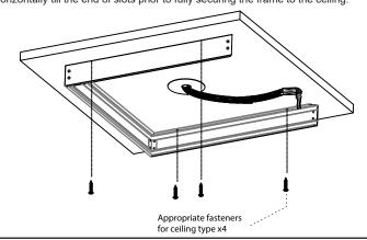
5.Put the wire conduit hose as close as possible to the surface mount opening before placing/inserting the luminaire into it partially.Make all electrical connections according to local code and make sure wire conduit hose is long enough for wiring connection in
