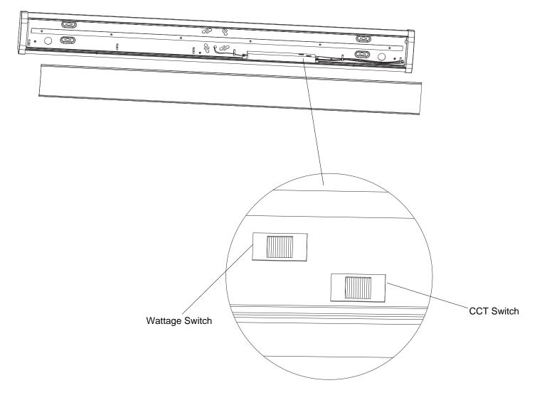
The end users may adjust the color temperature and lumen output respectively by the two DIP switch buttons integrated into the driver. Each DIP switch is accommodated with 3 options (left, middle and right ),corresponding to 3 color temperatures and 3 powers respectively, which can perform the desired color temperature and lumen output combination.
