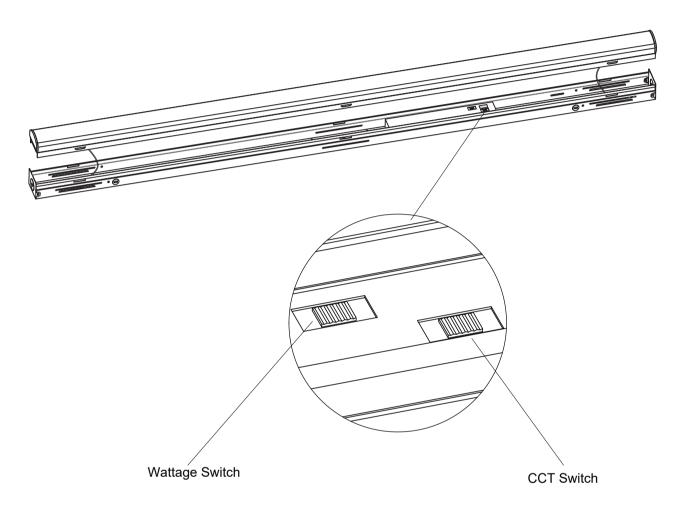
The end users may adjust the color temperature and lumen output respectively by the two DIP switch.Each DIP switch is accommodated with 3 options (left, middle and right ),corresponding to 3 color temperatures and 3 powers respectively, which can perform the desired color temperature and lumen output combination.
