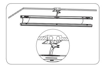
2.Fix the baffle on the lamp.
