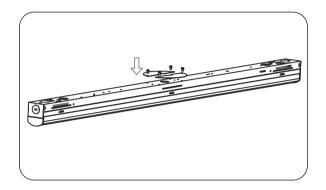
4.Fix the lamp to the ceiling with the plastic sleeve and screws provided.
