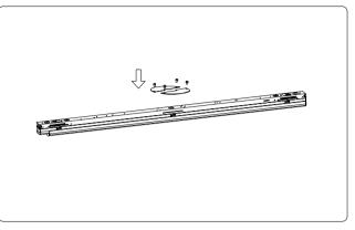
4.Mount the fixture to the ceiling with the plastic anchors and screws
