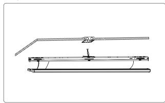
6.Assemble the module board upwards. The installation is completed.
