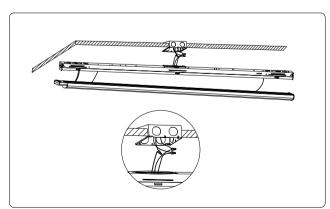
2.Attach the adapter plates to the back of the fixture with screws.
