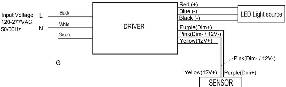
1. Dimming wires to 0-10V IEC compliant control.
